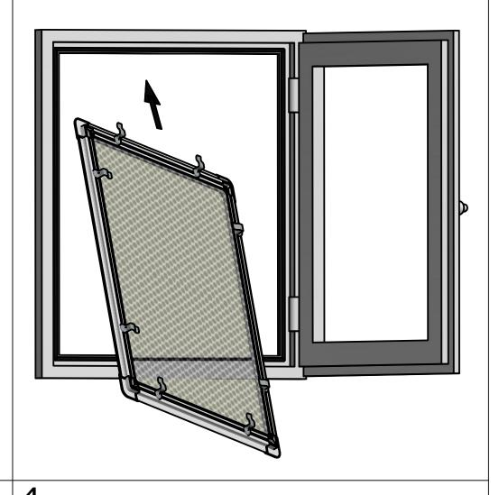
Attach the upper clips, located behind the mosquito screen, to the window frame lip. Then, holding the screen, attach the remaining clips and press it down to the frame.
